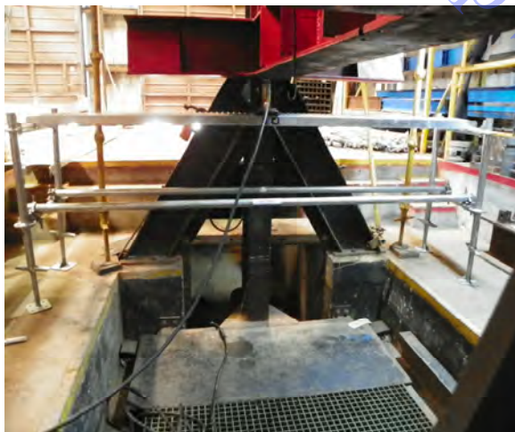
10' point load setup
