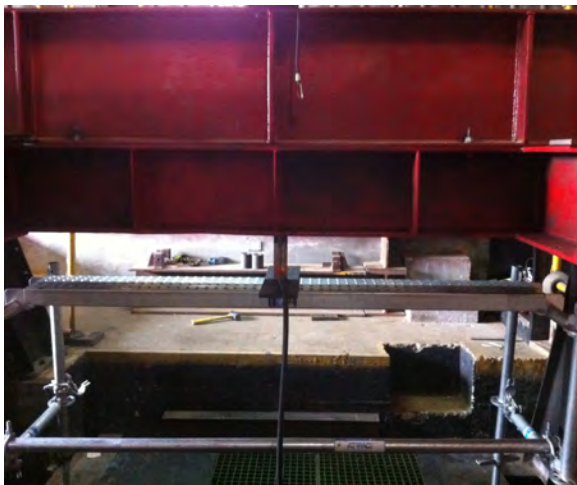
7' point load setup
